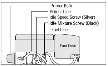
Figure 15: Idle Mixture Screw can be adjusted.
